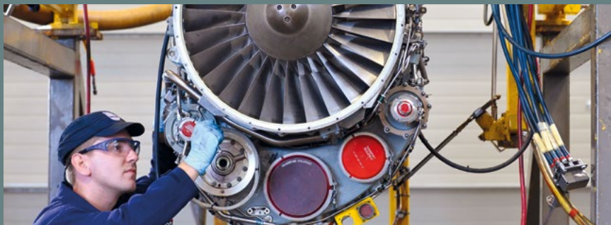
Critical maintenance of Hawk jet turbine
