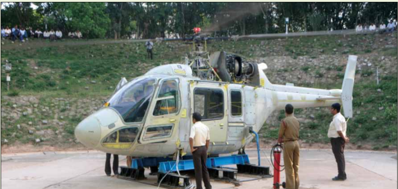
HAL successfully carried out the first Ground Run of Ground Test Vehicle (GTV) of Light Utility Helicopter (LUH) on 6 th December, 2014.
