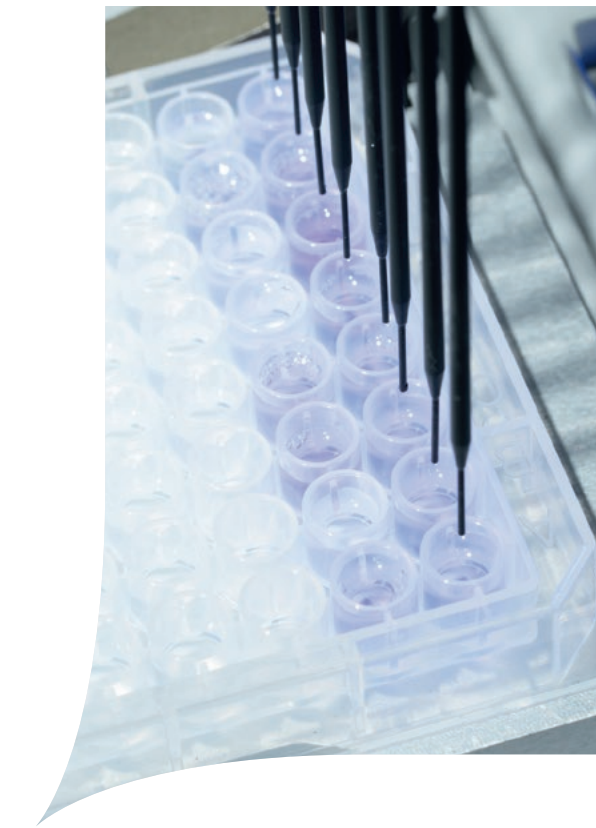
Automated 96-well-plate sample preparation. © P. Avavian/CEA
