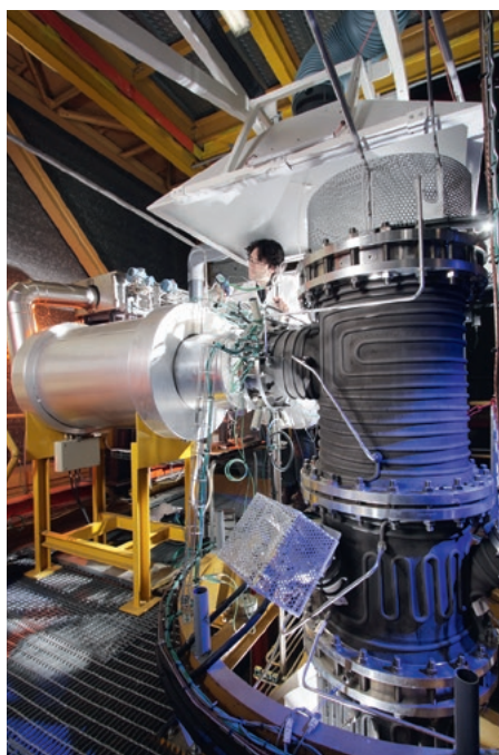
Pegase facility designed to host thermal biogas purification. © P. Avavian/CEA
