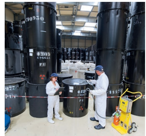
Checking the radiological condition and conformity of radioactive waste packages. © L. Godart/CEA
