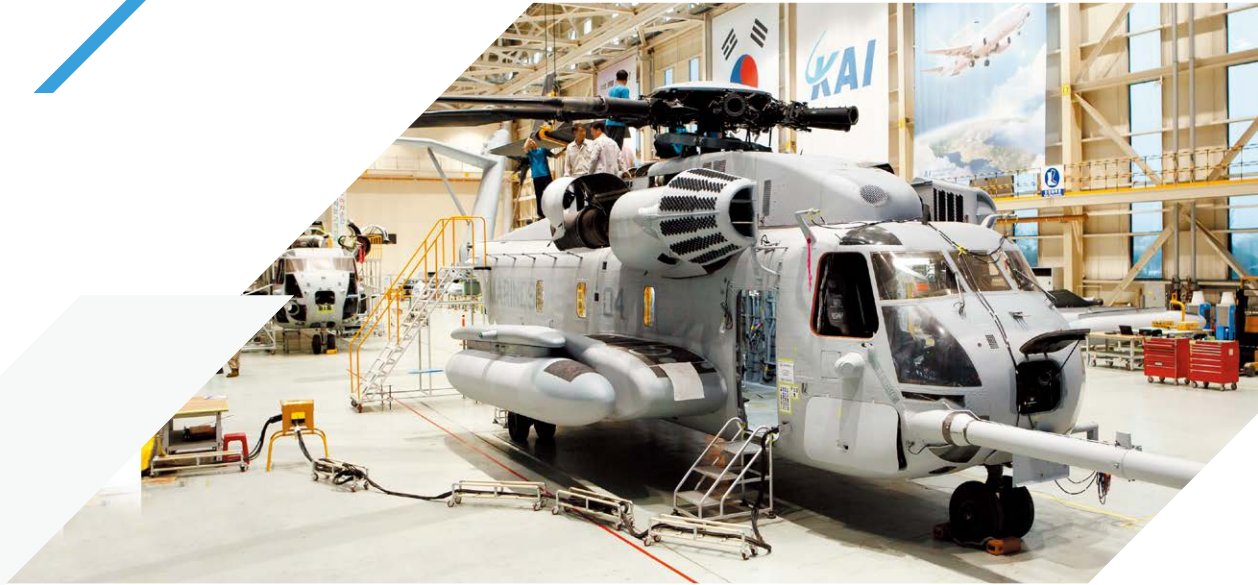
H-53 : Helicopter in operation by the US Navy and Marines for heavy-lift / long-range transportation, mine detection and removal, and search and rescue
