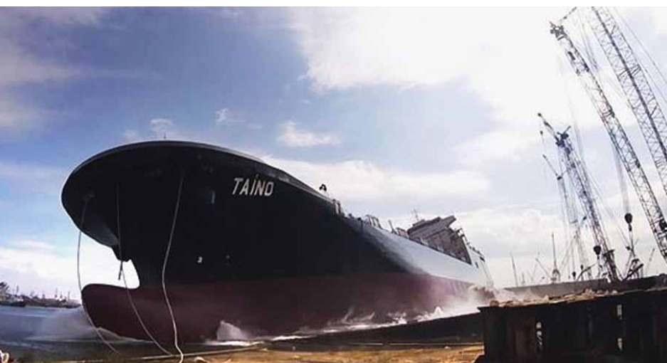
El Taino is the first American-flagged LNG-powered Container Roll-on/Roll-off ship.
