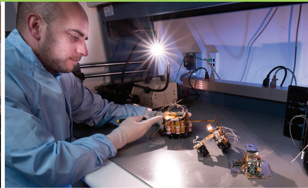
➤ Aerospace's Geoff Maul assembles the avionics components for AeroCube 7.
