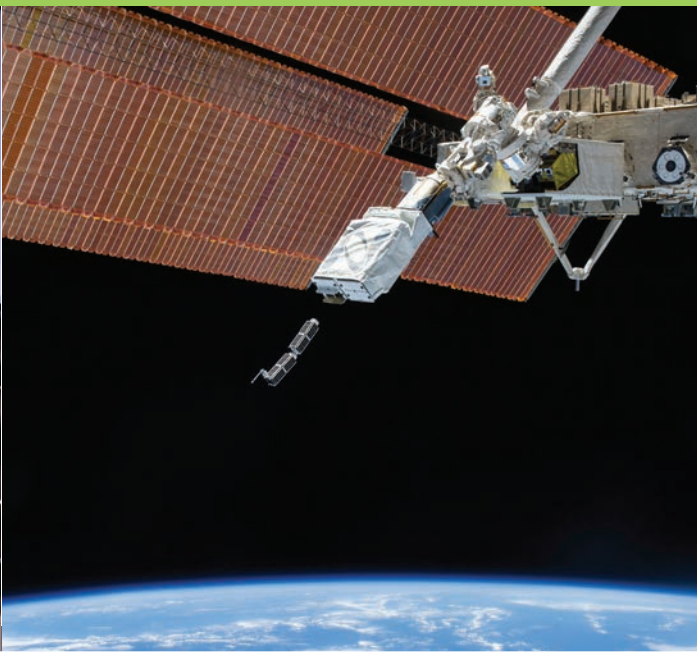
⤴ The Small Satellite Orbital Deployer, in the grasp of the Kibo Laboratory robotic arm on the International Space Station. (Photo courtesy of NASA)
