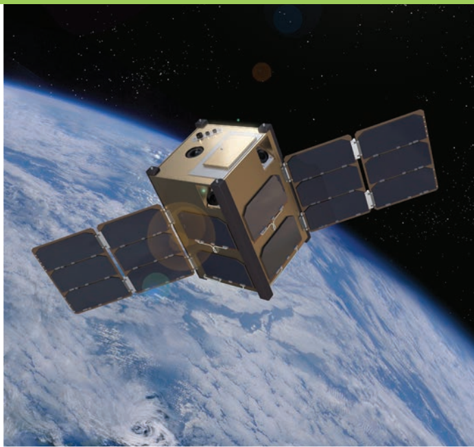
⤴ Artist's illustration of one of the CubeSats Aerospace is designing for a NASA-funded mission to study the upper atmosphere.
